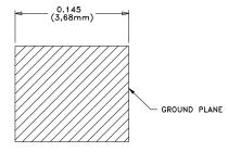
Unless Otherwise Specified: TOLERANCE: X.XXX = ± 0.005 DIMENSIONS APPLY BEFORE SOLDER ALLOW 0.015 MAX FOR PRETINNED SURFACES
