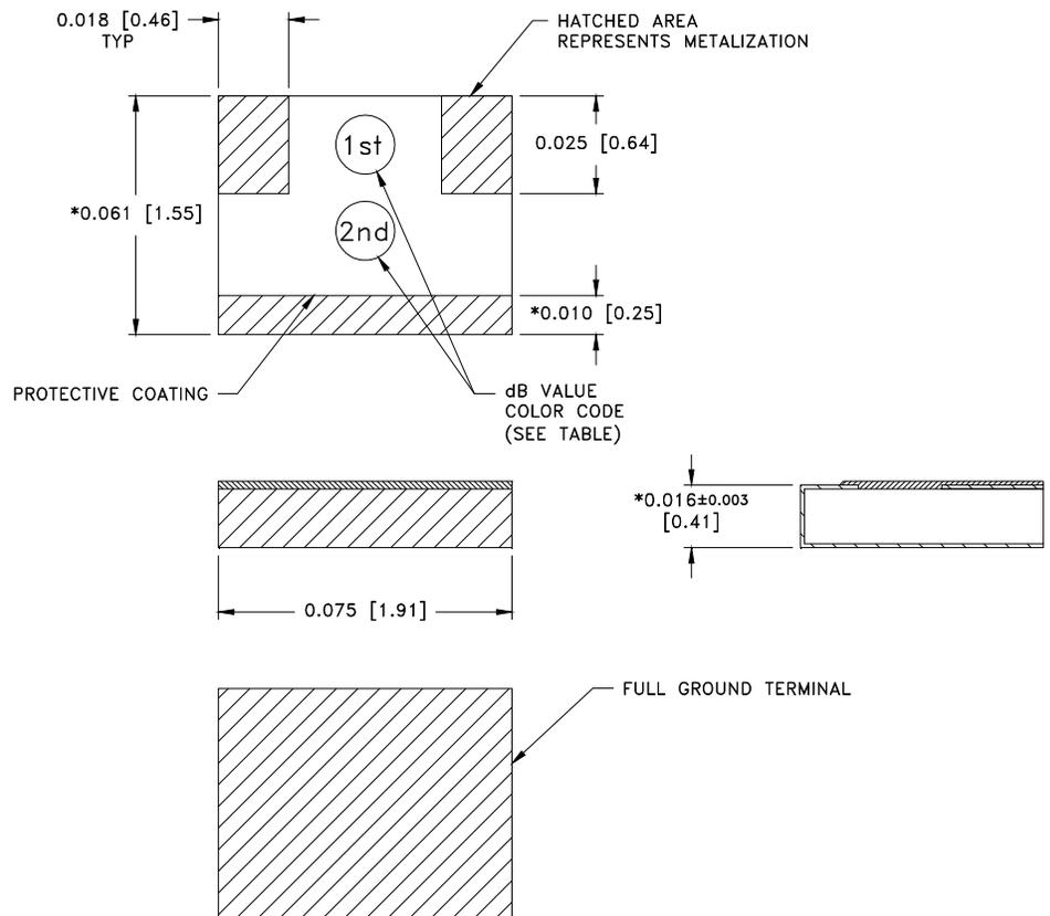
\* DIMENSIONS APPLY BEFORE SOLDER. ALLOW 0.015 MAX FOR ALL PRETINNED SURFACES.
