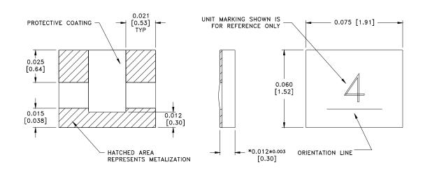
\* DIMENSIONS APPLY BEFORE SOLDER. ALLOW 0.015 MAX FOR ALL PRETINNED SURFACES.
