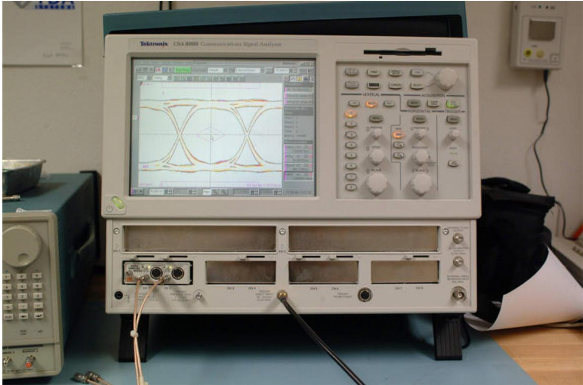
**Figure 6 The Tektronix CSA 8000 with 80E04 Sampling Head**
