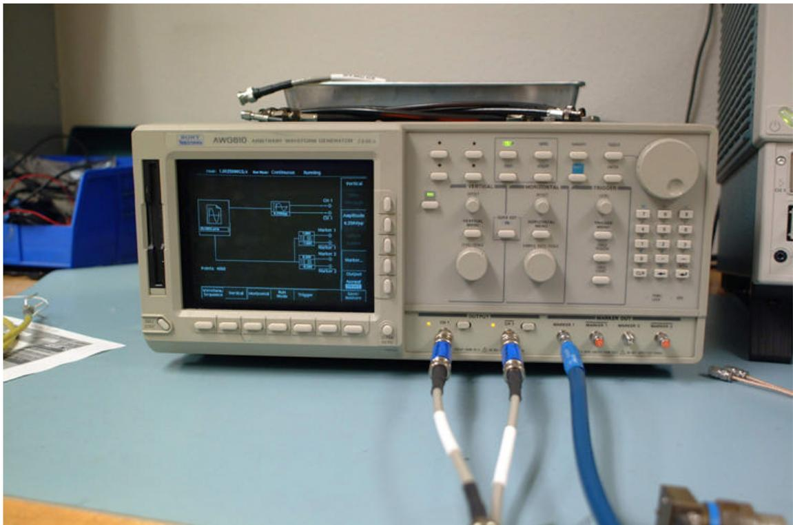
**Figure 7 The AWG 610 Arbitrary Waveform Generator**
