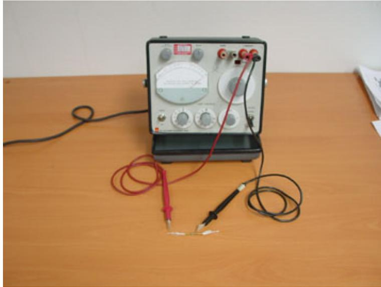
**Figure 4 Insulation Resistance Test Set Up.**
