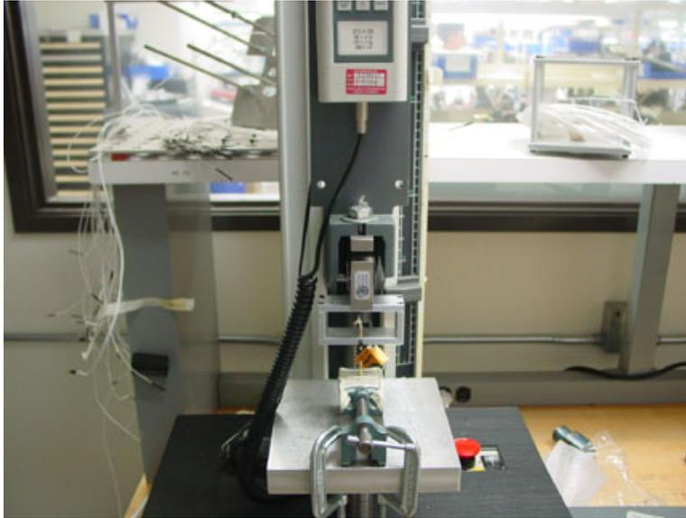
**Figure 3 Contact Engagement/Separation Force Test Set Up.**
