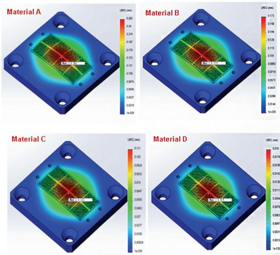
Figure 5: Spring probe head bowing in FEA.
