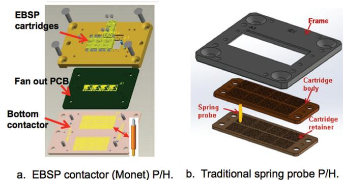
Figure 1: Typical structures of spring probe heads.
