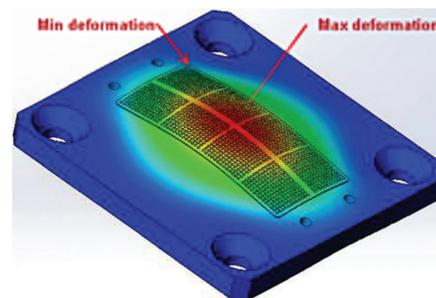
Figure 7: Maximum bowing in the center of the probe head center.
