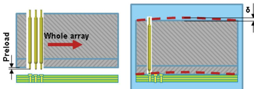
**Figure 4:** Spring probe preload and probe head bowing.
