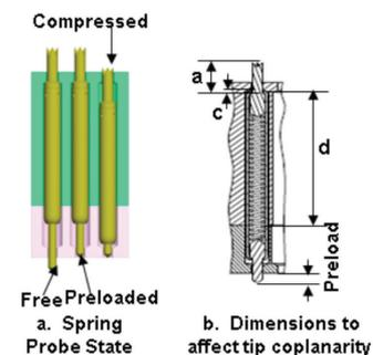
Figure 2: Spring probe state and dimensions that affect coplanarity.
