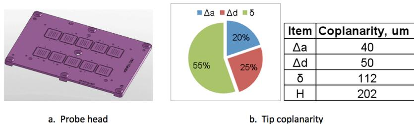
**Figure 3:** Example of spring probe head tip coplanarity distribution.
