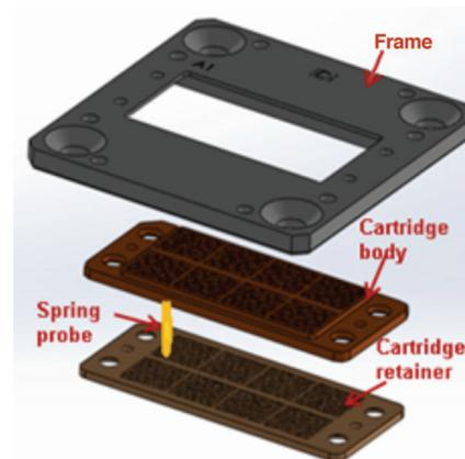
Figure 8: Probe head with frame.
