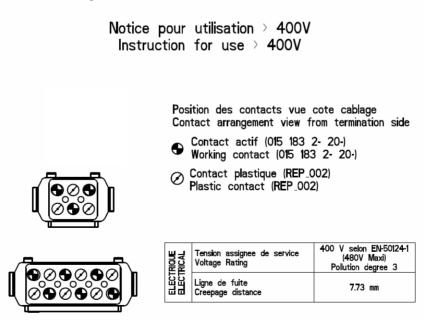
For use at 400V, the cables used must comply with EN50264-2-1
