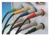
Incorrect mating also can be avoided by using keyed connectors. These incorporate a mechanism that physically prevents the plug and receptacle from being mated if they are an unmatched pair.
